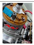
Rok Mini: Tech seal wire should run through the head nut and wrapped around the cooling fin. (One drilled nut required).
